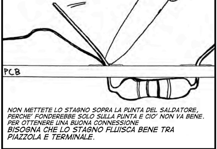
NON METTETE LO STAGNO SOPRA LA PUNTA DEL SALDATORE, PERCHE' FONDREBBE SOLO SULLA PUNTA E CIO' NON VA BENE. PER OTTENERE UNA BUONA CONNESSIONE BISOGNA CHE LO STAGNO FLUISCA BENE TRA PIAZZOLA E TERMINALE.
